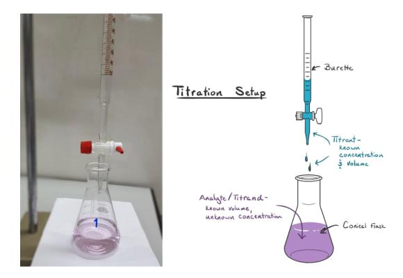
As part of the 'quantitative topic' in Chemistry, Upper 5 pupils have been carrying out titrations. Titrations are used to find the unknown in a neutralisation reaction. When an acid and alkali react together, a specific concentration and volume of each is required. Typically, the volume of the acid required is the unknown which the pupils had to use calculations to work out.
