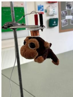
Lower 6 pupils have recently been studying the equations of motion and how to apply these to projectile motion. Last week they carried out the classic 'monkey and hunter' experiment. A hunter fires a projectile at a monkey that drops from the branch as soon as it hears the sound. Where should the hunter aim? Up, level or down? Using their knowledge of projectiles, pupils successfully hit the monkey with a ping pong ball.
