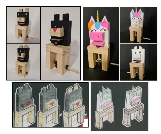
Last term in design technology, Lower 4 pupils have been diving into the fascinating world of cams and motion mechanisms. As part of their project, they explored how cams are used to convert rotary motion into linear motion and how these principles can be applied creatively.
